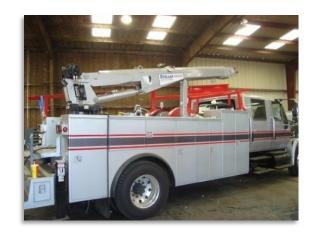
Wireline truck accessory options include multiple size drum draw works to fit desired slickline and braided line sizes (split drum or double drum available).
