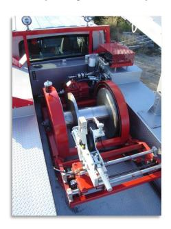
Drum wireline capacity is configured to customer requirements. Drum Drive Performs at a Drum Speed Up to 2000 fpm with up to 6,000 lbs of pulling power. Training/Commission of unit conducted at customer location.
