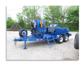
The winch hoist specifies a 3 & 4 speed Funk transmission, 2 speed hydraulic motor, machined & balanced drum, and open/closed-loop hydraulics. It is designed to be compact, yet accessible.
