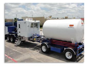
Precise uses only proven components such as ACD brand triplex, cold ends and liquid nitrogen centrifugal pumps. Manual, electrical and pneumatic valves are utilized. Autoclave and Butech type high pressure 316 & 304 stainless steel lines. 2500 to 3000 gallon liquid nitrogen storage vessel are available.
