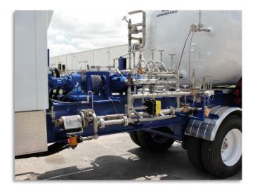
The Precise control panel is sectioned by operating process. Included in all panels are real time pressure and flow data recording with on board job storage and laptop charting. Stainless steel panel with all unit controls. Data Acquisition Systems available upon request.
