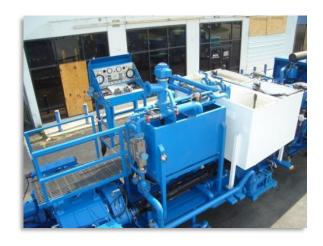
Precise utilizes the time proven RCM mix system. The system is designed electric over hydraulic for infinite control of the slurry delivery system. Micro-Motion fluid densitometer is utilized for precise customer product delivery. Fully computerized mixing system available upon request.
