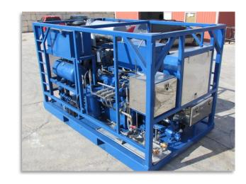
Major Components include a Liquid Nitrogen Pump, Model GUPD triplex reciprocating cryogenic pump with 1.625" Bore Size and 1.5" Stroke, "POT" type Vaporizer, and Diesel Engine Heat Recovery System designed to convert engine heat and waste system heat into useful heat for Nitrogen vaporization. Also includes Engine as specified by customer, Liquid Nitrogen Charge Pump, and Liquid Nitrogen Centrifugal Pump Model 1½ x 2½ x 6.
