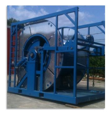
All connections are Aeroquip. Includes 3.06 Bore Quad BOP and Side Door Stripper. Complete unit assembled and tested for customer acceptance at Precise Energy Products' facility in Ft. Worth, Texas. Training / Commission of unit conducted at customer's location. Data Acquisition Systems available upon request.
